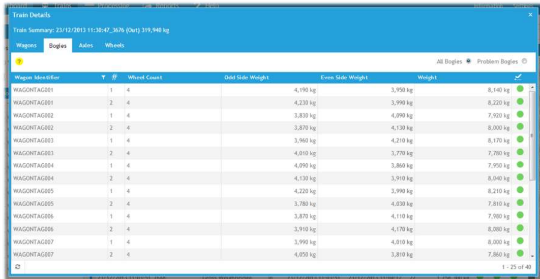
Figure 8: Train Detail, Bogies Screen
